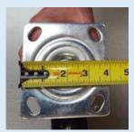
Measure the *top plate* by locating where the caster will be attached and the top plate that will be used. To do so, measure the outside to the outside of the top plate one way (length) and then repeat this on the perpendicular side (width).
