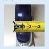
The **diameter** is measured with the wheel lying flat on its side, and with a measuring device measure from one side of the wheel to the opposite side. Make sure the measuring device passes over the center of the wheel. To measure the **width**, stand the wheel upright and measure from the outside of one side to the outside of the other.
