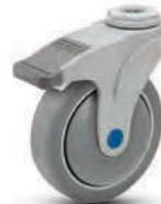
Our Directional Lock casters are designed to lock the swivel but not the wheel allowing you to steer your equipment. The directional lock feature is designed to break free under heavier load when the unit is traversing a corner only to lock back into position when the unit resumes a straight course.
