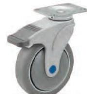
Our Directional Lock casters are designed to lock the swivel but not the wheel allowing you to steer your equipment. The directional lock feature is designed to break free under heavier load when the unit is traversing a corner only to lock back into position when the unit resumes a straight course.
