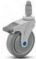
Our Directional Lock casters are designed to lock the swivel but not the wheel allowing you to steer your equipment. The directional lock feature is designed to break free under heavier load when the unit is traversing a corner only to lock back into position when the unit resumes a straight course.
