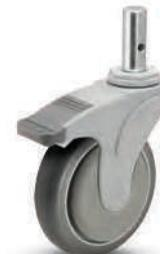
Our Directional Lock casters are designed to lock the swivel but not the wheel allowing you to steer your equipment. The directional lock feature is designed to break free under heavier load when the unit is traversing a corner only to lock back into position when the unit resumes a straight course.
